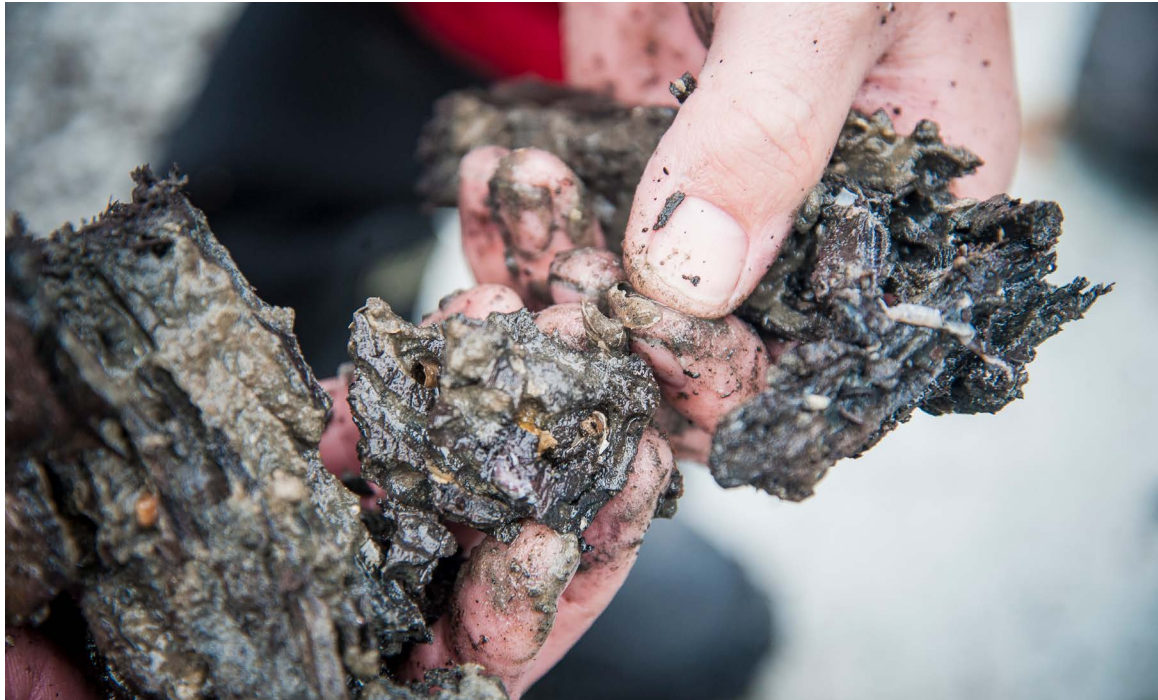
^ Fig. 6 Previously-strong, hard oak wood from a shipwreck in the Wadden Sea (the Netherlands) has crumbled and almost disappeared due to the attack of the shipworm ( Teredo navalis ) (Source: Cultural Heritage Agency of the Netherlands).
