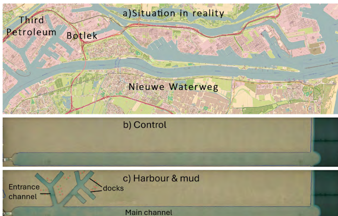
^ Fig. 4 a) Situation of the Nieuwe Waterweg and setup of the straight channel with harbors in the Metronome (sea is on the right side in the images; Metronome is 20 by 3 m) (Source: © OpenStreetMap contributors, 2024. Open Database License, ODbL v1.0); b) Control; c) Harbor and mud setup schematic representations (Source: Authors, 2025).
