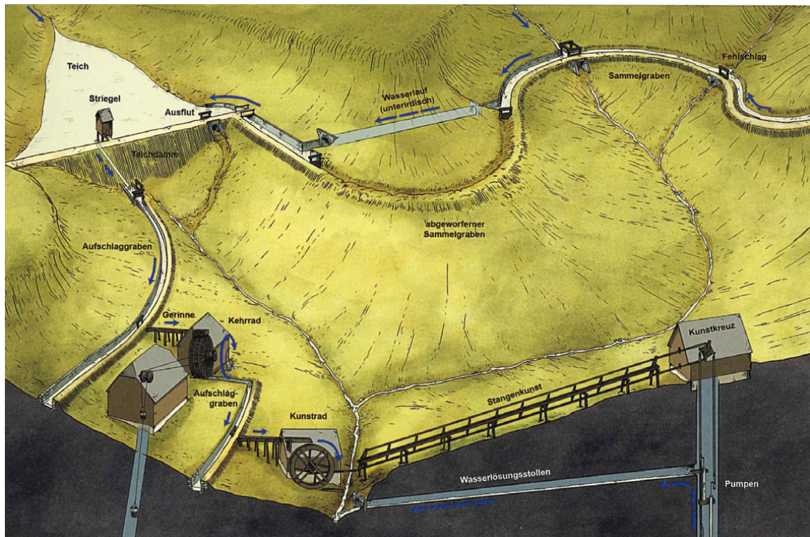
^ Fig. 2 Functional diagram of the Upper Harz Water Management (Source: H. J. Boyke in the 1990s, colored by J. Bintakies in 2013).
