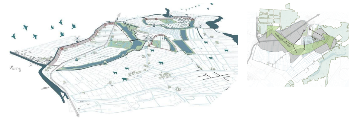
^ Fig. 12 Birdseye view of the Polder Renewing project showing the three lake-bed polders (-4.5 m NAP) with the newly implemented inner-boezem landscapes and two additional water storage basins in the peat polder landscape (-1.5 m NAP). The basins are connected, creating an ecological corridor (Source: Jingwei Gua and Chenye Yang, 2023).
