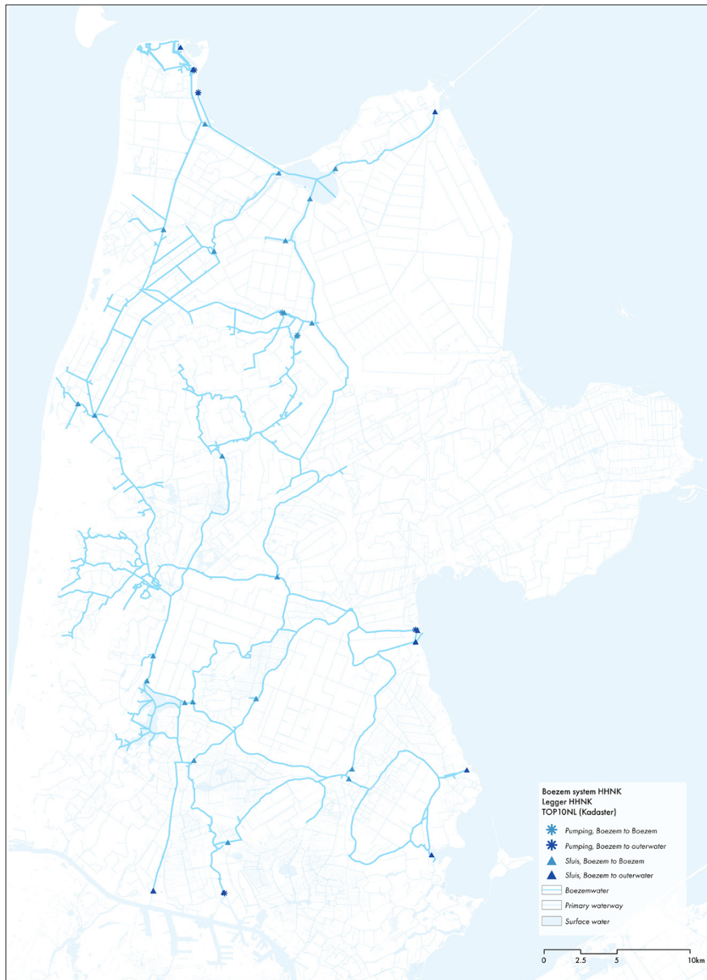
^ Fig. 2 The polder-boezem system of North-Holland above the Amsterdam-Rhine Canal. Water from the polders is discharged by pumping stations (not depicted on the map) into the boezem system, from which it is subsequently conveyed through boezem pumping stations toward the outer water: to the north into the sea, to the east into the IJsselmeer and to the south into the Amsterdam-Rhine Canal (Source: Inge Bobbink and Michiel Pouderoijen, 2016. Based on TOP10NL (Kadaster) maps from HisGIS, Fryske Akademy © HisGIS open data, www.hisgis.nl ).
