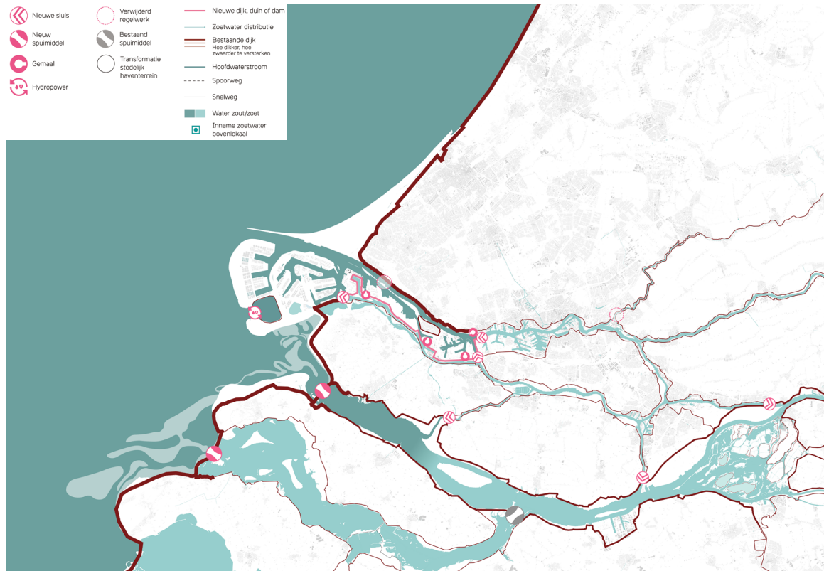
^ Fig. 11 Polder strategy showing main river discharge via the Haringvliet, with a dam at its mouth. The Nieuwe Waterweg will also be closed by a dam. The existing flood defense system, indicated in red, will be enhanced (Map: De Urbanisten, 2026; source: IABR Delta Rijnmond-Drechtsteden 2100).
