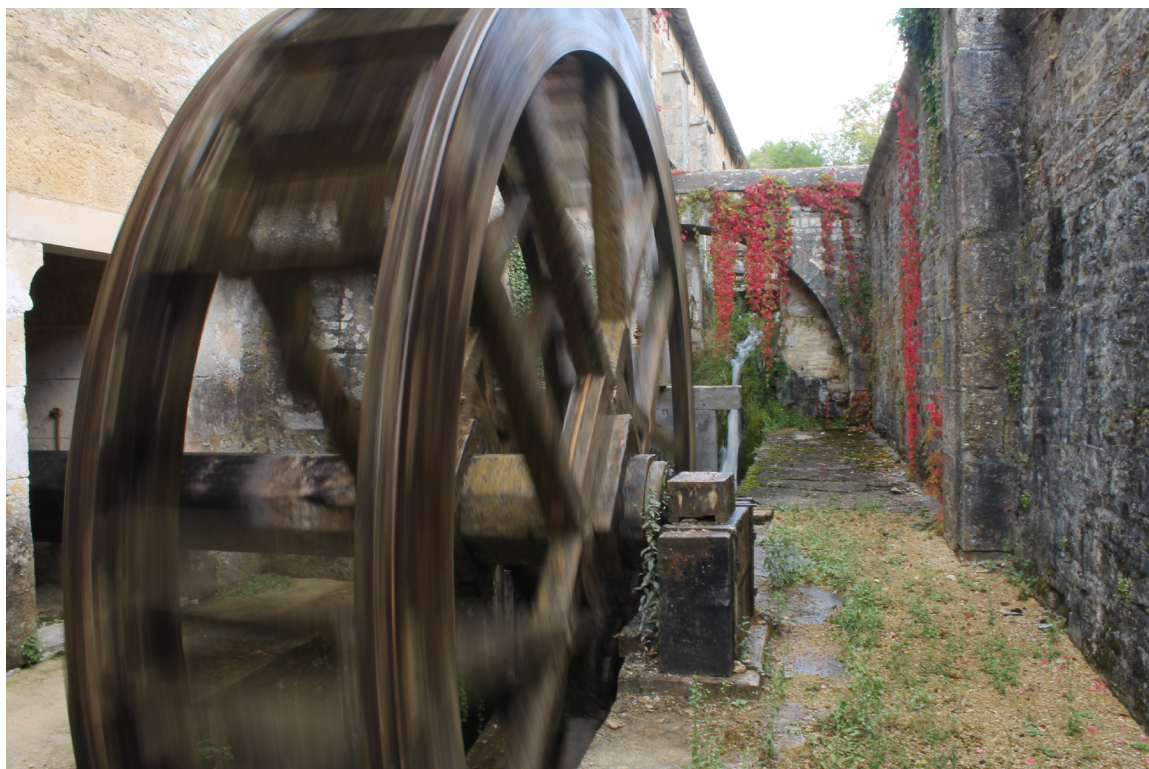
^ Fig. 3 Abbey of Fontenay – UNESCO Monastic Site, France. Hydraulic wheel driving the trip hammer in the Cistercian forge, illustrating medieval monastic water management and the integration of technology and spiritual life within a self-sufficient economy (Source: Draceane, 2013. CC BY-SA 4.0, via Wikimedia Commons).
